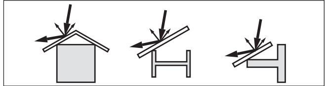
Fig. 11: Cover flat, large-area profiles with deflectors
